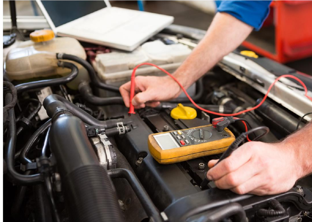
Figure x.x. Easy testing with the TMX 301 Reader. The handheld leads on the TMX 301 reader allow you to easily test various engine components.
